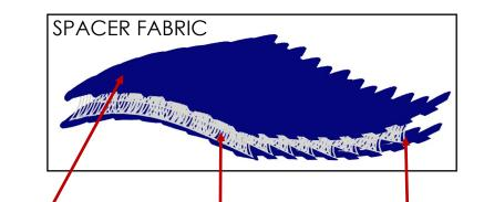
**OUTER LAYER PROVIDES FIRST** LAYER OF FILTRATION.
